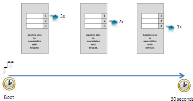
Figure 3.1 Switching to static IP address
